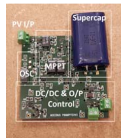
3. Energy Harvester & Graph of Efficiency vs. Supercap Voltage
