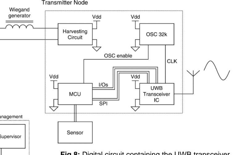
Fig 8: Digital circuit containing the UWB transceiver, MCU, oscillator and an external sensor
