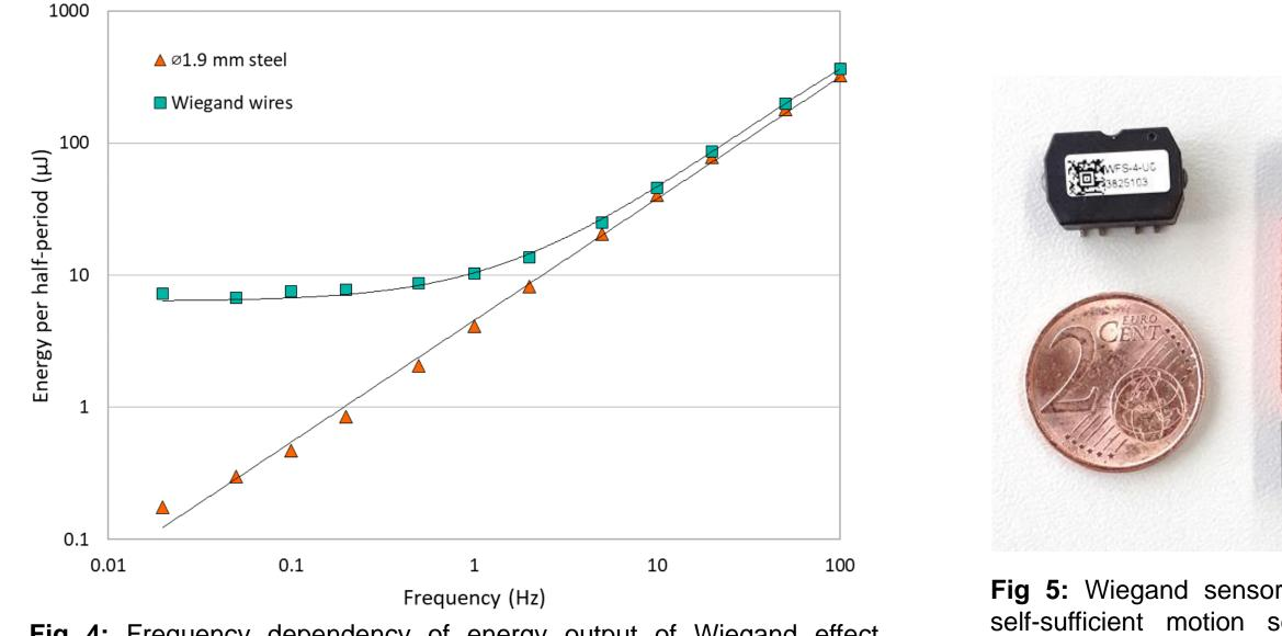
Fig 4: Frequency dependency of energy output of Wiegand effect compared to regular induction. Coil (8000 wdgs), oscillating field (16mT), Joule heating power in a 3 k $\Omega$  resistor measured.
