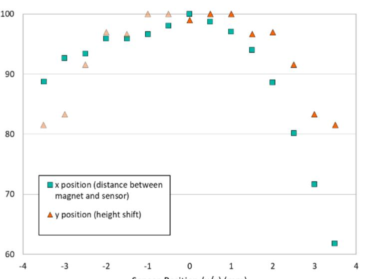
Sensor Position (x/y) (mm) Fig 6: Mounting tolerances of the magnets with respect to the Wiegand generator.
