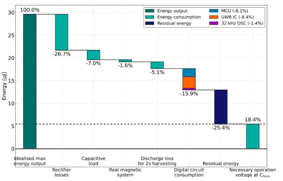
An average of 25.4 % (7.5 µJ) residual energy can be additional for sensor used MCU further readouts, calculation for stability and security or increased UWB payload data transfer.
